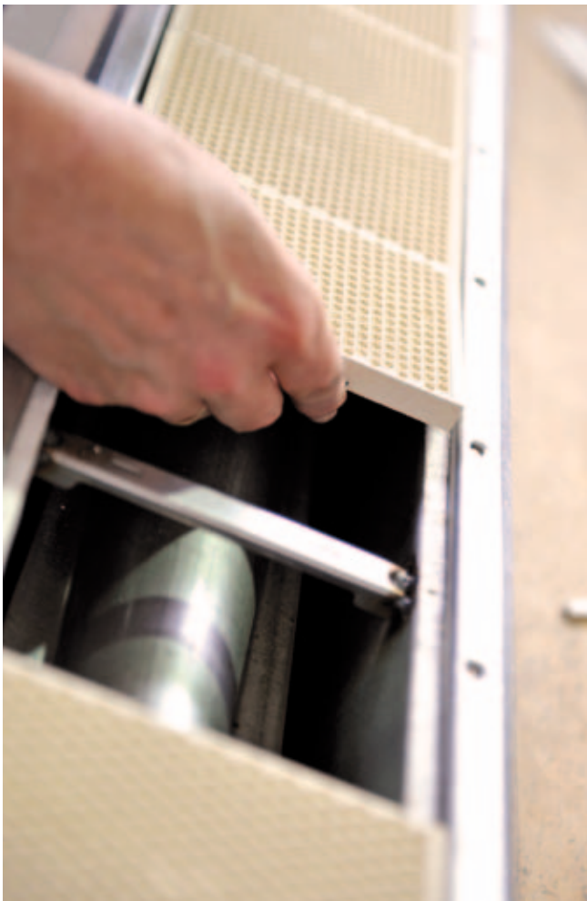
Lining of burners with ceramic tiles.
